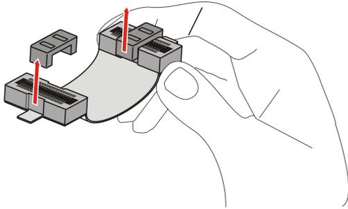
Figure 3–3 ATI CrossFireX Installation
